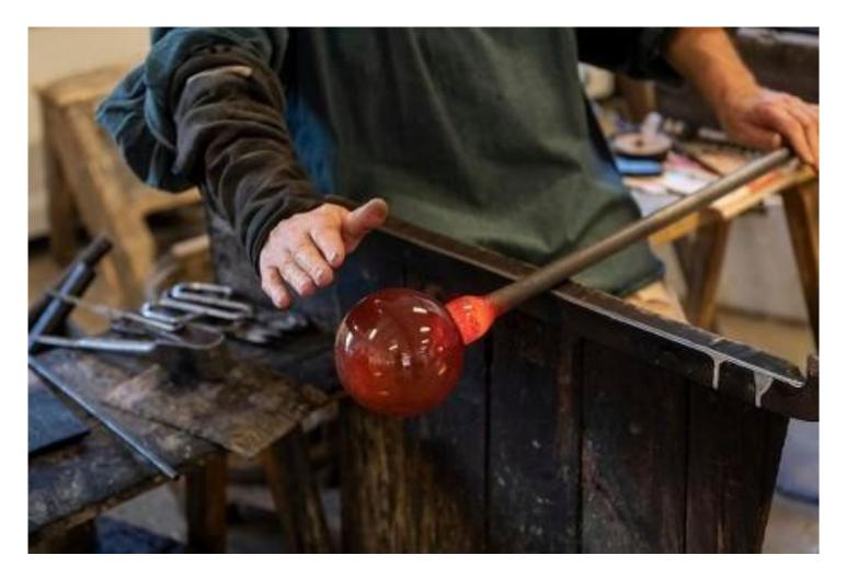
Glassblowing is an ancient craft that involves heating glass until it becomes soft and pliable, then blowing air into it through a pipe or tube to form bubbles and shaping it into various forms by hand or with the aid of tools.
